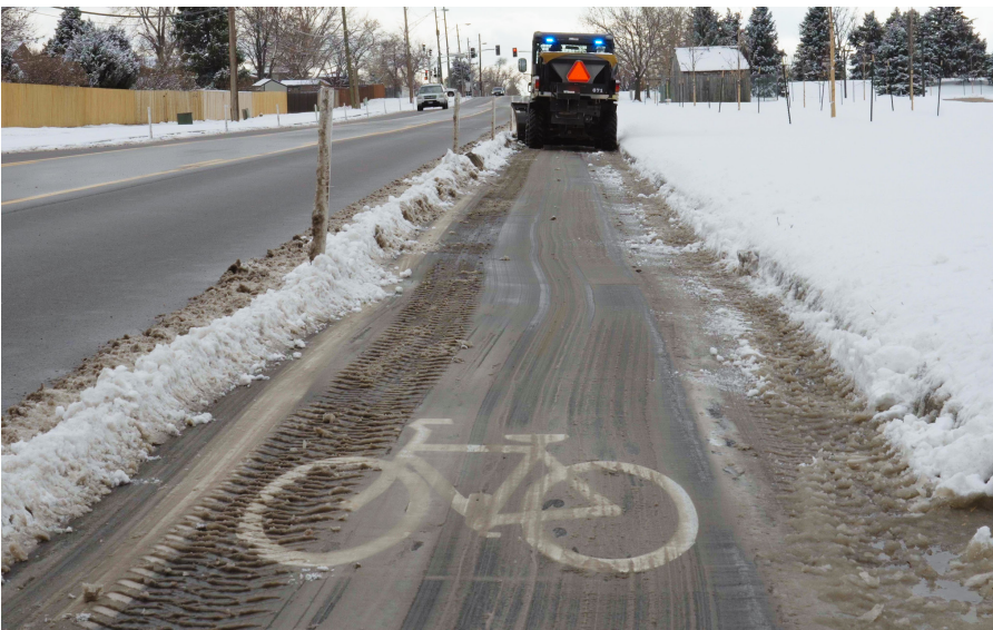
The Public Works Department uses scaled-down snowplowing equipment to keep Lakewood's new separated bike lanes on Garrison Street, Denver West Parkway and Harlan Street usable during the winter. For more information about snow clearing on shared-use paths and bike lanes, visit Lakewood.org/SnowPlan .
