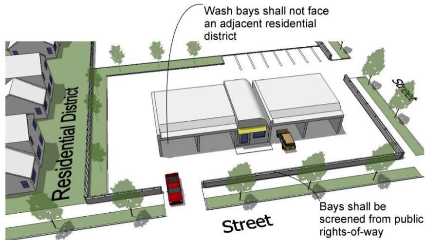
Figure 17.7.7: Car Wash Bay Location
